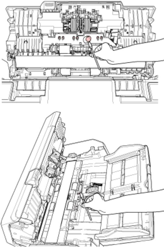
**5 Feed roller to be cleaned as you rotate the roller manually (× 2)**
