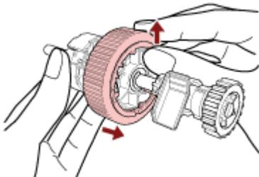
**7. Attach new pick rollers (× 2) on the shaft one by one.**
