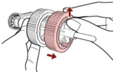
b. Pull out the other pick roller from the shaft as you lift the retaining clip.
