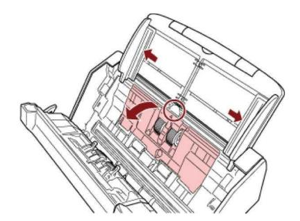
b Rotate the bushing in the direction of the arrow.
