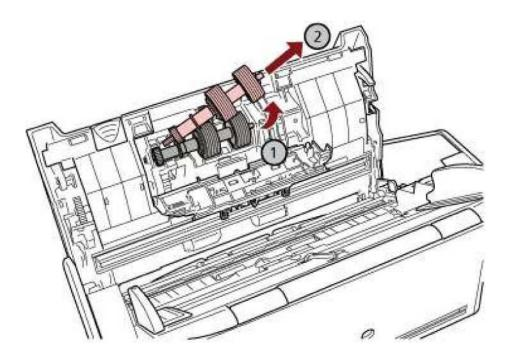
c Remove the brake roller from its shaft.
