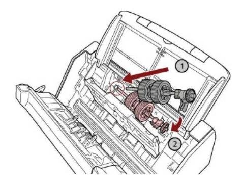
e Rotate the bushing in the direction of the arrow.
