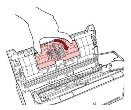
b Remove the brake roller.
