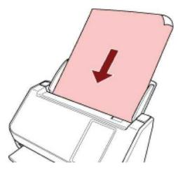
7 Adjust the side guides to the width of the Cleaning Paper.
